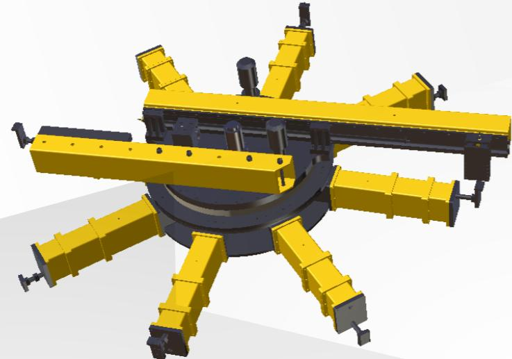
FI3000 Flange Facing Machine adopts the disk type high precision slewing bearing support structure, relative to the spindle structure, the anti-overturning moment of the equipment is enhanced, and the overall height of the equipment is greatly reduced, especially the aseismatic ability of the tool arm is enhanced during vertical processing.
