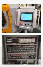
tton. Press the emergency stop button to cut off the power supply in an stop working. At the same time, the automatic processing program has ction. When restarting, you can choose to continue processing or restart
